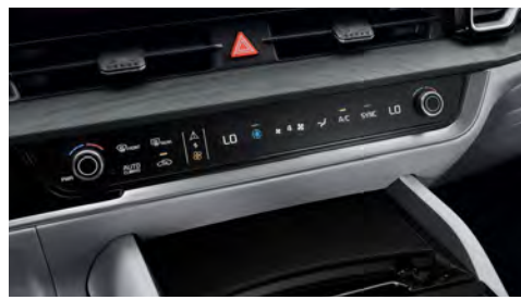
Infotainment/climate control system (includes the independently controlled full auto air conditioning system)
